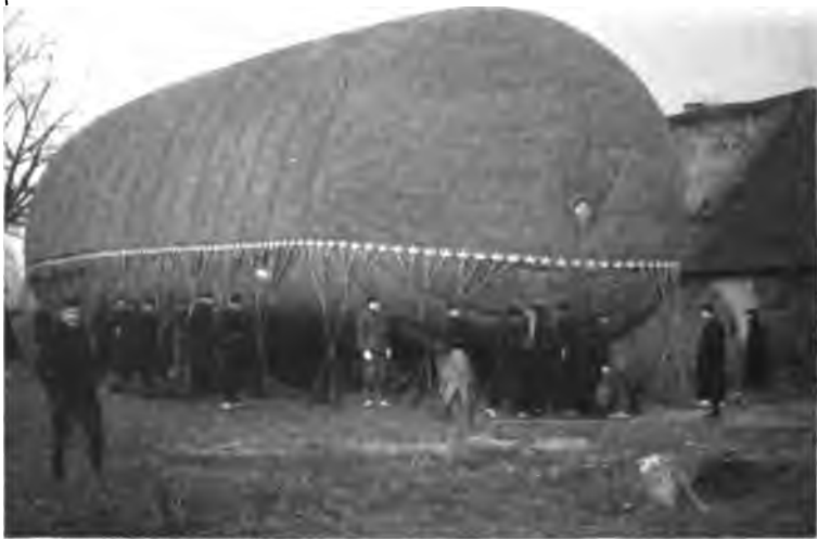
An observation balloon in service with the Belgian army. It is held to the ground by heavy weights until the observers are ready
